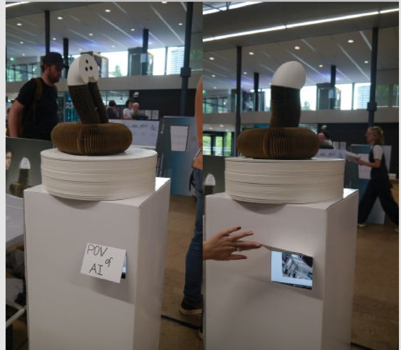
Image 41: Demoday stand of the project “Motion and Emotion“. The neck of the robot kept dismounting or tilting sideways. The base where the electronics were was not integrated with the rest of the stand.
